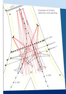
"The main advantage of the Frankfurt RIAS concept is the automated "safety net" – an intelligent set of sensors positioned in key areas of the airfield to detect critical situations that could lead to an actual incursion. When an event is detected, the system simultaneously alerts the responsible air traffic controller and the pilot/driver of the respective aircraft or vehicle."
